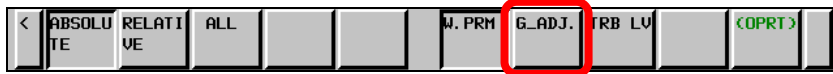
Fig.19.4.1 (h) Soft key to select trouble diagnosis graphic screen (10.4-inch display unit)
