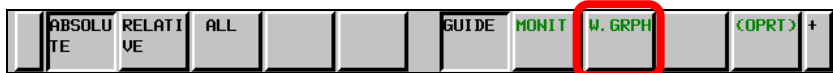
Fig.19.4.1 (e) Soft key to select trouble diagnosis graphic screen (10.4-inch display unit)
