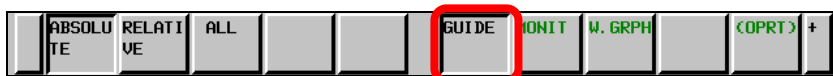
Fig.19.4.1 (b) Soft key to select trouble diagnosis guidance screen (10.4-inch display unit)
