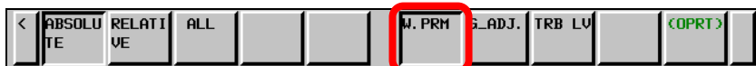
Fig.19.4.1 (f) Soft key to select trouble diagnosis parameter screen (10.4-inch display unit)
